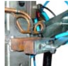
Copper cooling plates
